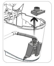
3. Remove fixing block and gasket
