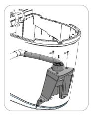
2. Loosen the three screws
